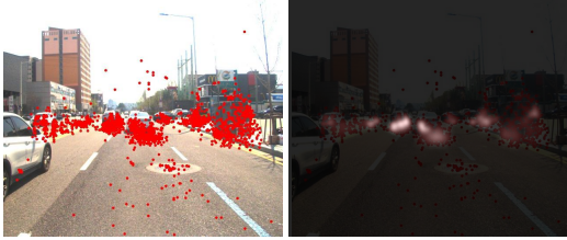
Fig. 5: Left: radar signal (red dots) projection on image, and Right: the corresponding signal distribution function illustrated in the grayscale image (translucent).
